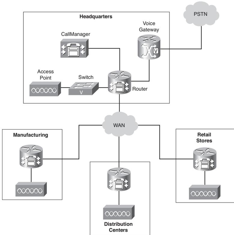
This system enables wireless VoIP communications among all of Acme Furniture's facilities. In addition, users can place and receive telephone calls from the Cisco 7920 IP Phones with standard telephone users via a gateway connection to the PSTN.
