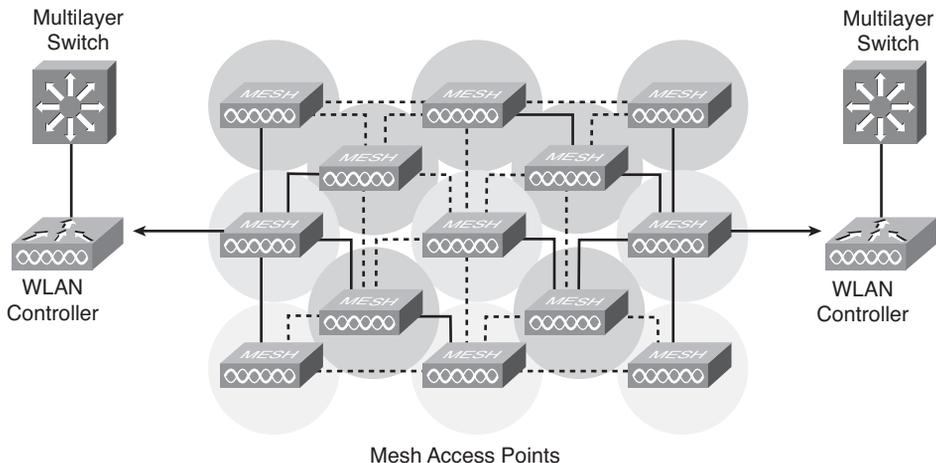
The operation of a mesh network is fairly straightforward. For example, the URL request from a Wi-Fi user enters the mesh network at the backhaul node that the user associates with using Wi-Fi protocols. Then it hops from one node to the other until it reaches the node that connects to the Internet service provider (ISP). In some cases, the data packets may hop only a couple of nodes, but a greater number of hops may be necessary in larger networks.
